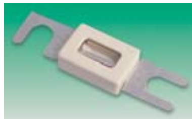
L (overall)=82, L (body)=32, W=22, H=10, Fixing centres=60, Lug spacing=11
